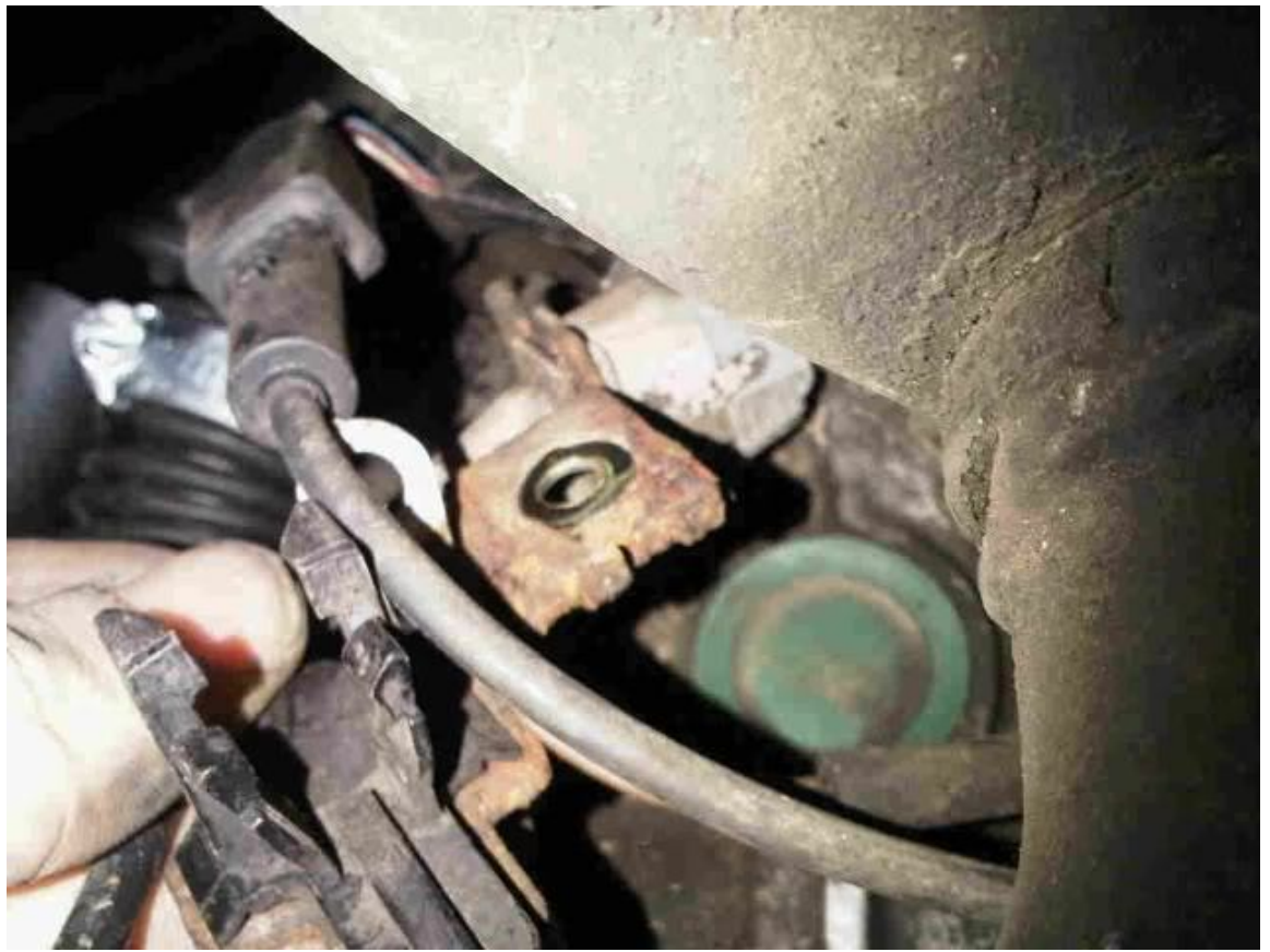
Disconnect hall sensor plug from bracket
