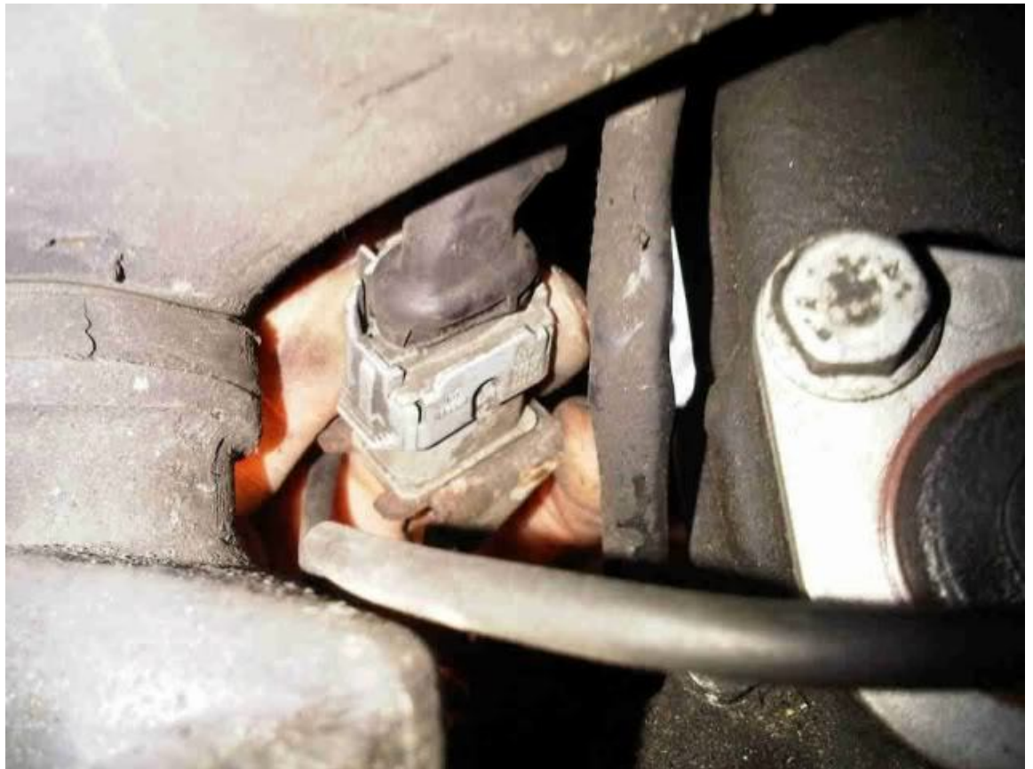
Remove sensor, clean bracket up if required
