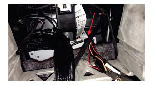
3.5 mm AUX terminator- must be fitted to cars original AUX port (if equipped)
